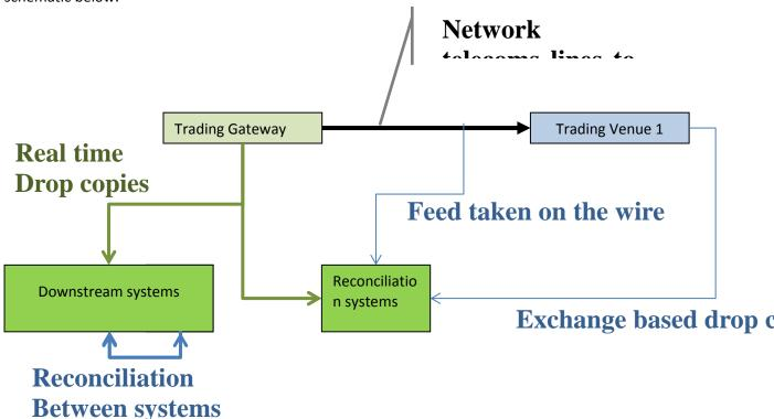
Instead of a drop copy, a feed can be "tapped" or "spanned" directly from the telecom lines, which then can be processed and compared to the information help into the trading gateway. This would achieve the same result than a drop copy provided by the exchange.
